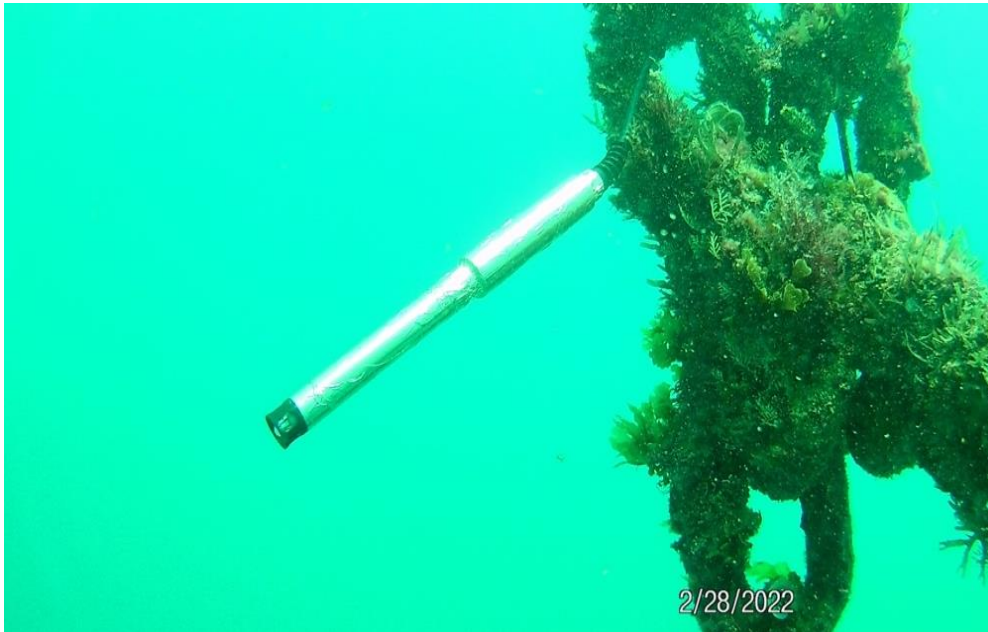
Aqualabo PHEHT sensor to measure seawater pH Source: Aqualabo and Digital Twin Services - © 2022
