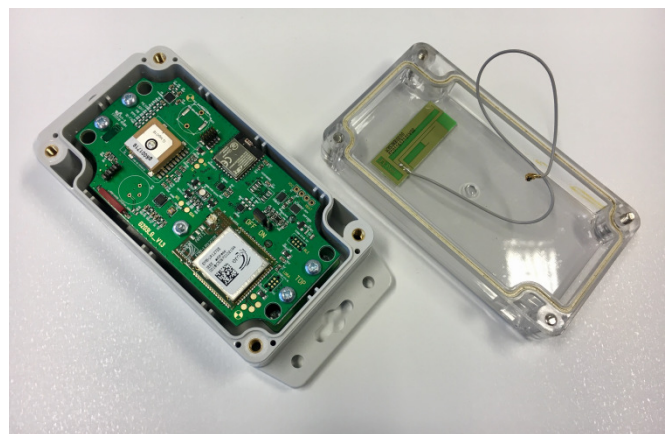
Photo 3: Conbee HybridTAG L500 (top view with removed cover)
