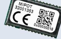
Thanks to its small LCC form factor (15.5  $\times$  26 mm only) and its low current consumption, this module allows the
