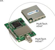
The mDot and xDot are LoRaWAN compliant,
