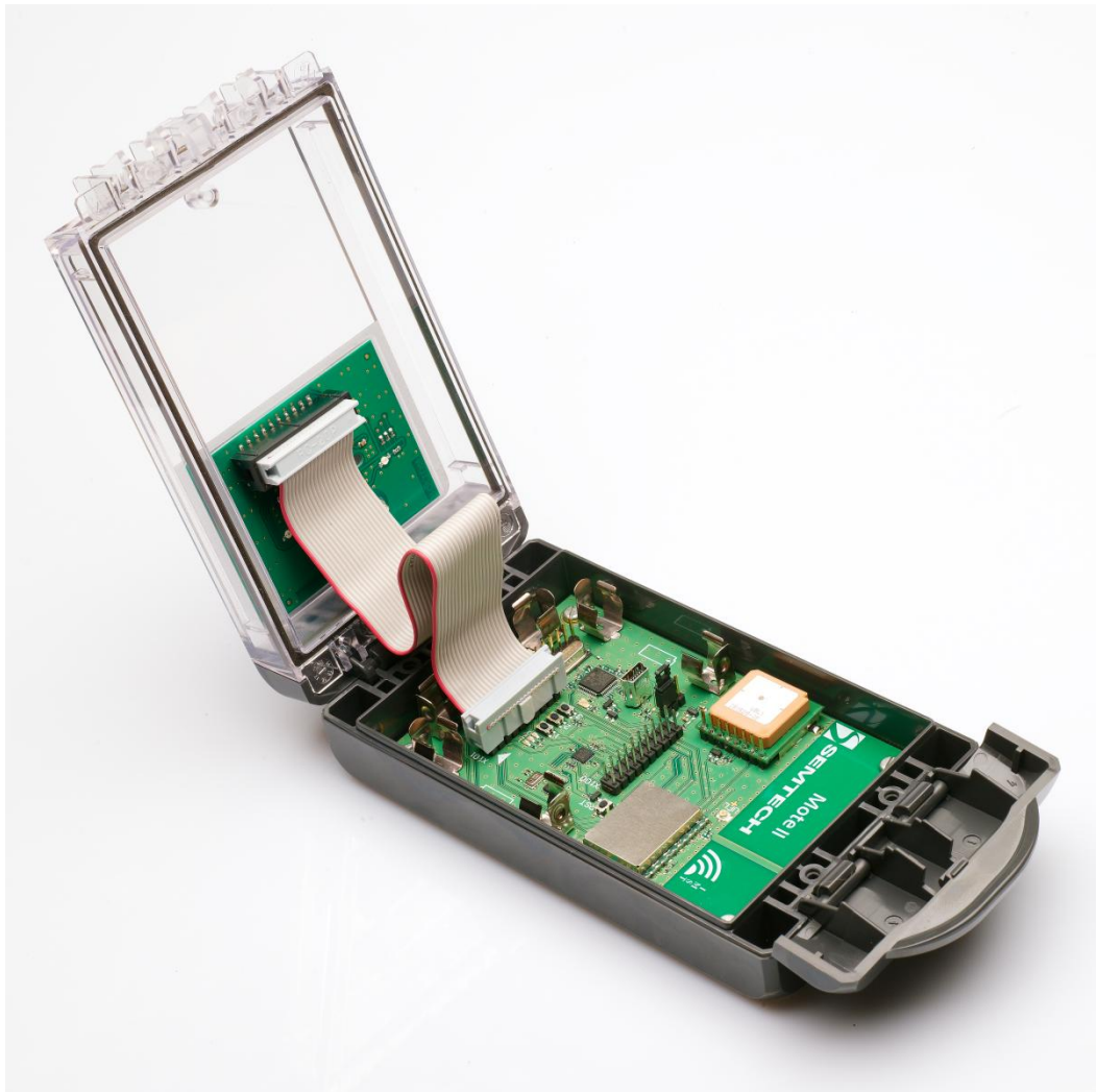
Figure 3-1: Mote II with open Cover
