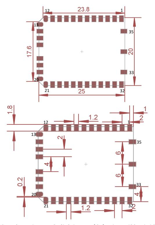
**Note:** Do not place any via or exposed pad in the inner area of the footprint to avoid short circuit between the via on customer board and the via on the bottom side of the EtherLoRa
