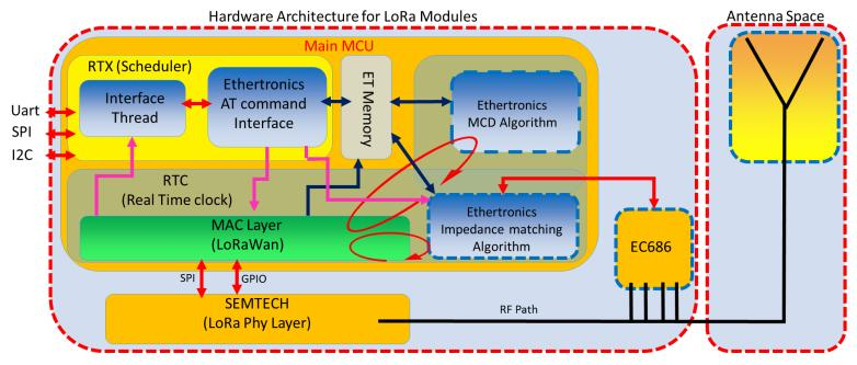
In this configuration, a proprietary impedance matching algorithm helps to maximize the power transfer to the antenna Please refer to the application note about the passive evaluation board for more details [4].
