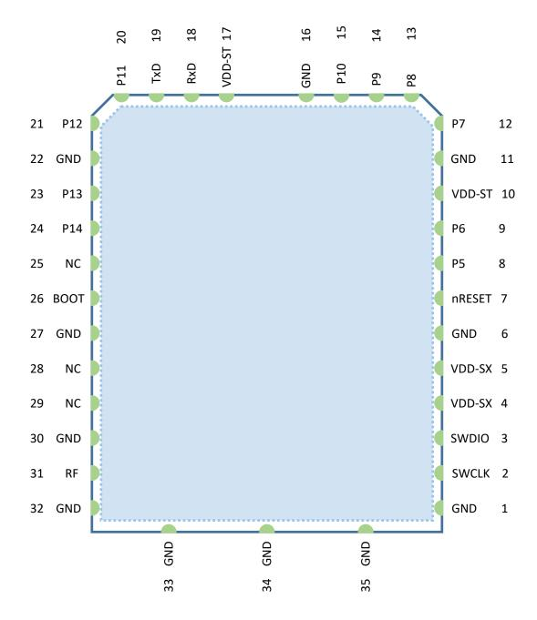
**Note:** Do not place any via or exposed pad in the inner area of the footprint to avoid short circuit between the via on customer board and the via on the bottom side of the ETH-LORA-M-AX-01
