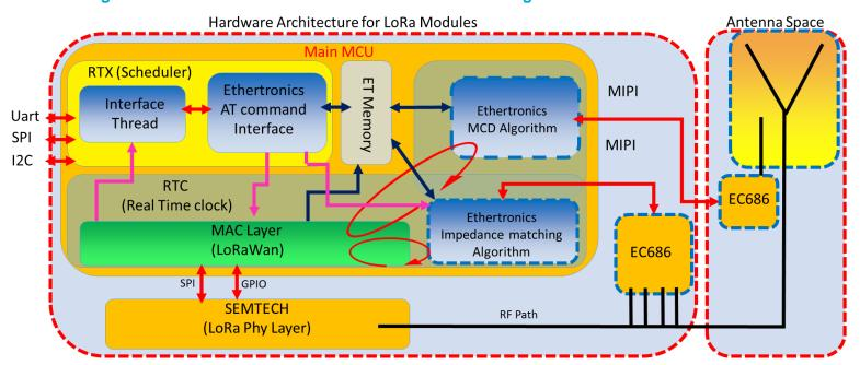
In this configuration, an active antenna with several radiation patterns must be used. In addition to the impedance matching algorithm, the MCD algorithm helps to choose the best radiation pattern regardless to the change of environment. Please refer to the application note about the active evaluation board for more details [5].
