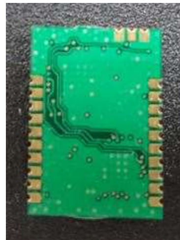
Photo 4: Radio module bottom view
