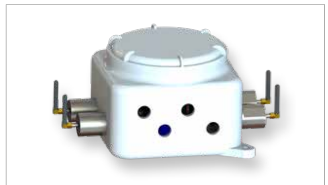
GUB EXD models for up to four transmitter applications ATEX rating: II 2 G Ex db ib mb IIC T6/T5 Gb II 2 D Ex tb ib mb IIIC T85°C/T100°C Db
