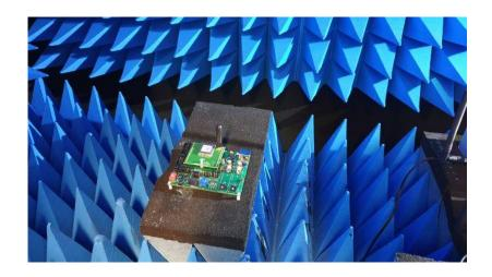
Figure 1 DUT Setup
