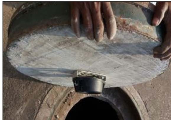
Level monitoring sensor under a manhole cover
