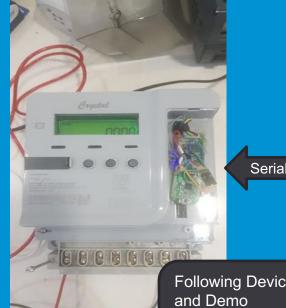
LoRaWAN Serial Module Secure Element
