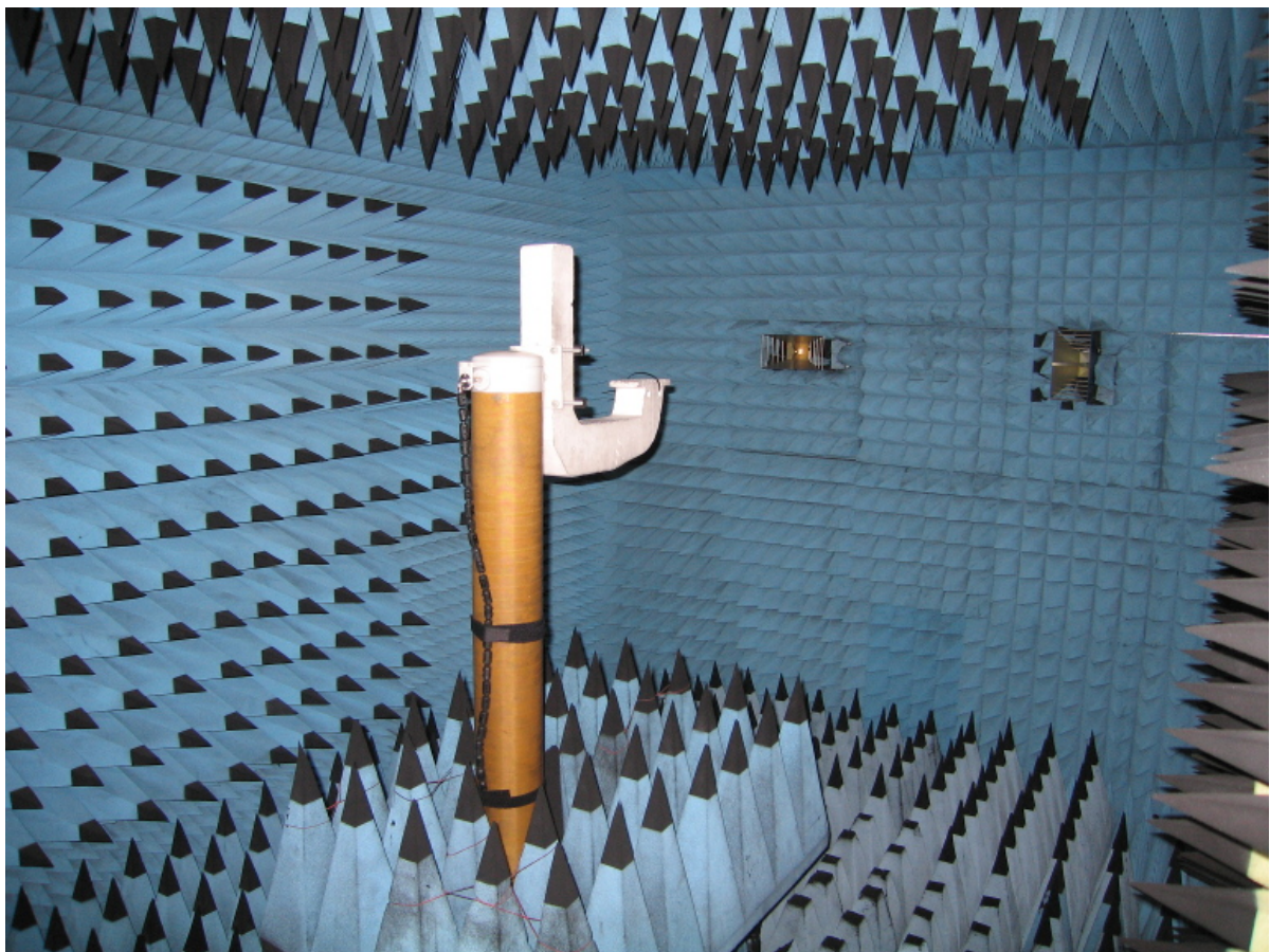
Figure 3.1: IMST Anechoic Chamber (Range II) B83117-A1431-T161
